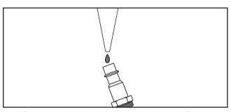
Figure 3. Lubricating directly into air fitting.
